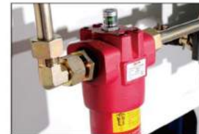
Germany imported HYDAC oil, the cartridge can be replaced
