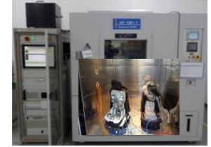
Seats are operated in the chamber @ - 40 ~ 120C to test switches
