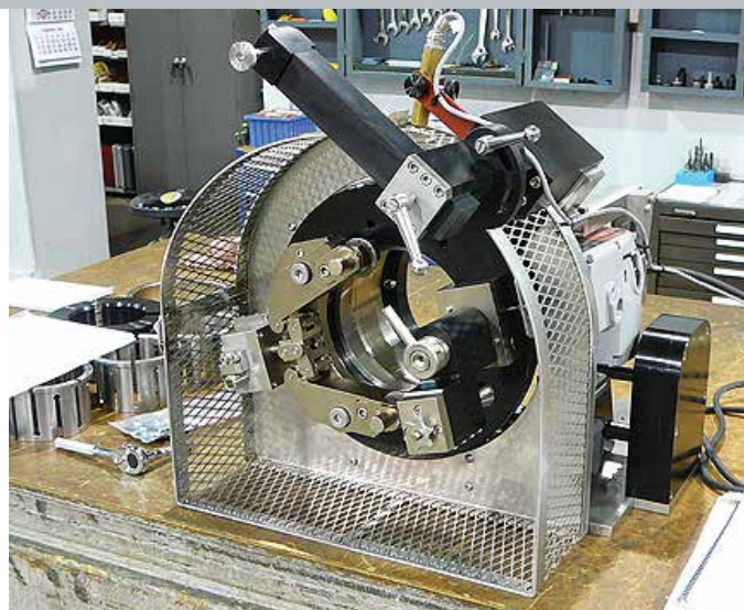
This 576 AC SeverMaster® was designed for use in a glove box. Configured with roller cutters, it performs remote chipless canister opening. Other unique features include a pivoting base stand, laser pointer for cut location reference and a burnishing module to push the burr out of the way to allow removal of the inner can.
