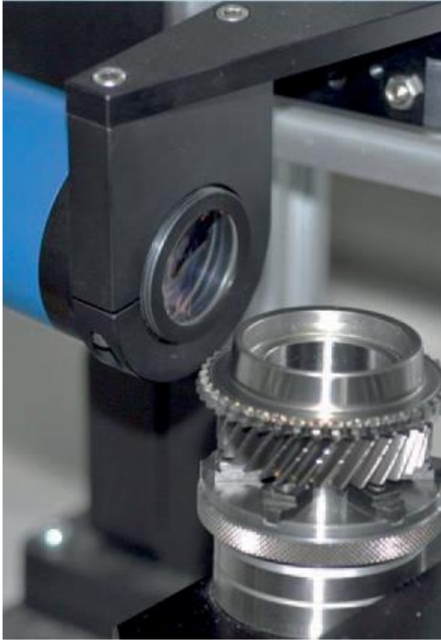
Roughness and roundness measurement on the control gear
