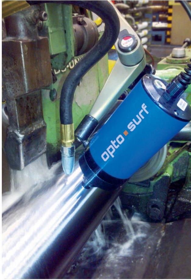
In-process surface measurement on rollers
