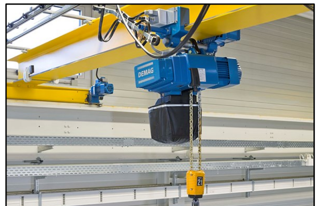
Overhead Trolley System
