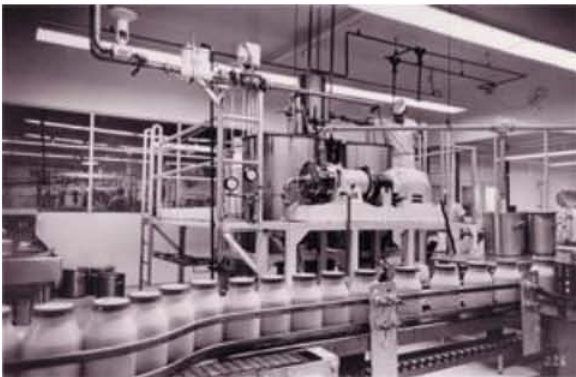
Typical Mayonnaise Plant using the Charlotte Continuous Mayonnaise Machine
