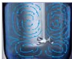
Eurostar mixer working principle
