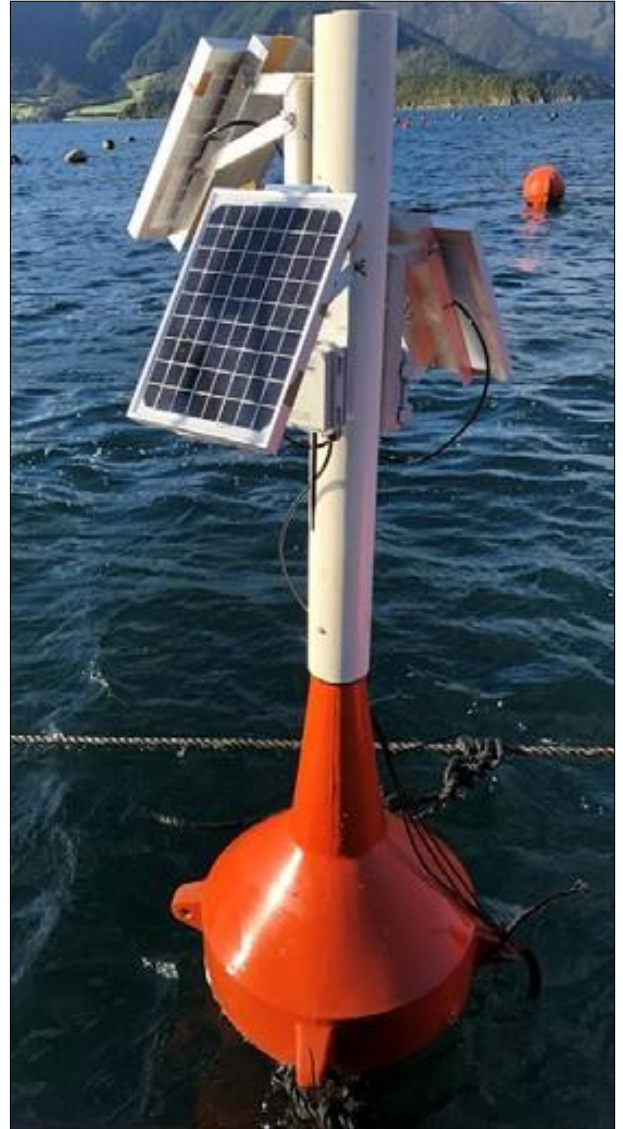
LoRaWAN-based water quality monitoring network at a Marlborough Sounds mussel farm, New Zealand.
