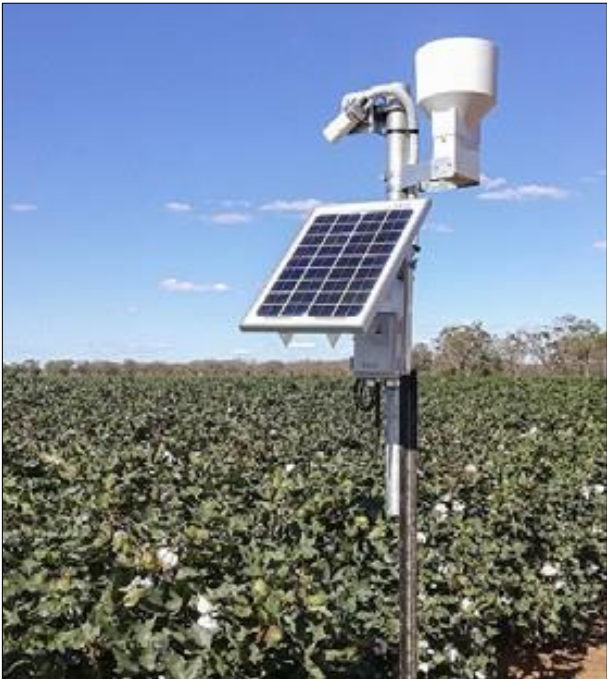
CWSI and Rainfall being recorded in Cotton and transmitted by LTE Cat M1/Cat NB1/EGPRS system - Narromine NSW
