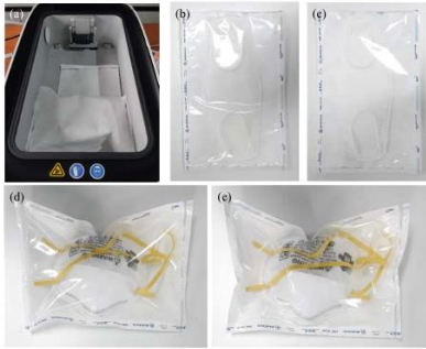
Figure 1.2 (a) The position of the masks sealed by Tyvek® pouch. The figure of (b, d) before and (c, e) after the sterilization for KF94 and N95, respectively.
