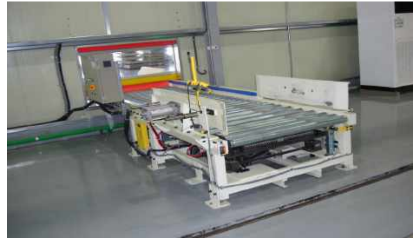
In-Out Let Conveyor System & Centering Device (3 ton)
